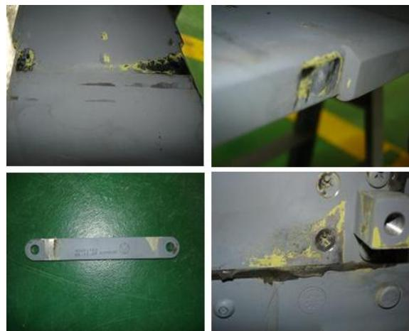
Fig. 6. Frictional wears on the strut components
