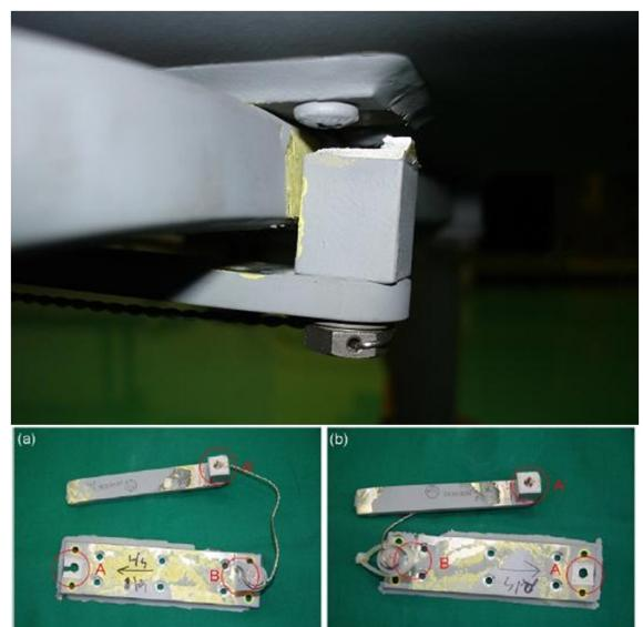
Fig. 2. Landing gear strut with the fractured lugs
