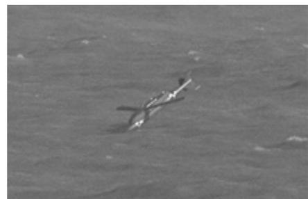
Fig. 5. Sea impact test with limited explosion
