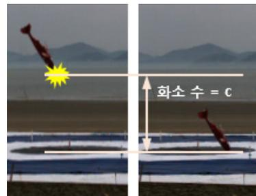
Fig. 9. HOB measurement of ground impact test
