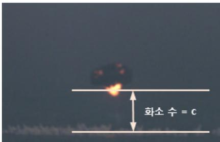
Fig. 4. HOB measurement of sea impact test
