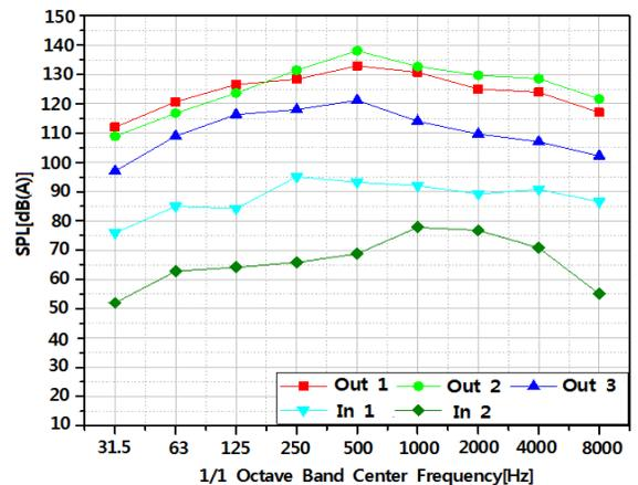
Fig. 7. The measurement value of the noise at inside and outside of the shelter
